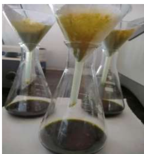
Fig.7. Filtered with whatmann filter paper
