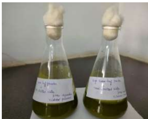
Fig.5. 50g guava leaf powder and 500ml distilled water in 2 flasks
