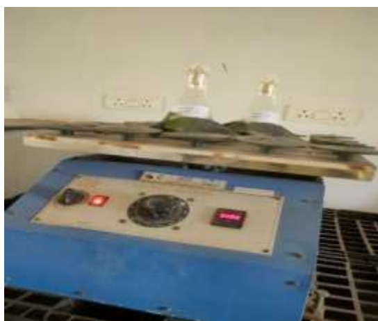
Fig.6. Kept on rotatory shaker at 160 range speed
