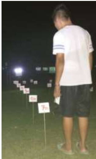
Step 9. Evaluation of lights activation from 1 meter to 7 meters within an angle of 60 degrees right
