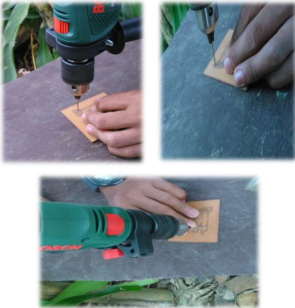
Figure 8. Boring holes for the placement of components
