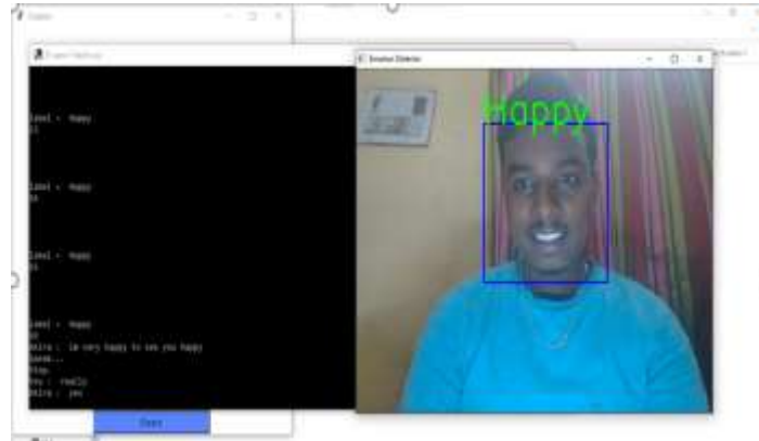
Fig 5: By selecting the speech option, the user can capture real-time face detection via webcam.
