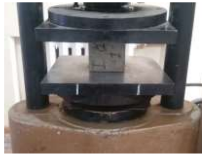
Figure 6. Concrete samples placed in molds and the process of testing the sample in a press: a) molding the sample; b) test the sample under the press.
