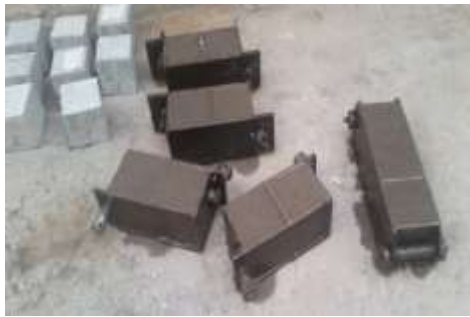
Figure 6. Concrete samples placed in molds and the process of testing the sample in a press: a) molding the sample; b) test the sample under the press.
