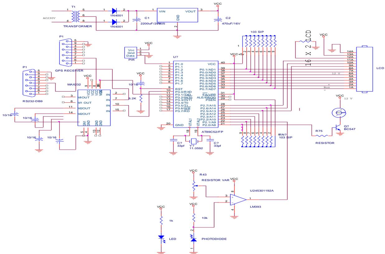
**Fig. 2.**Circuit diagram of human detection robot
